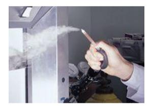
**Smoke tubes** can be used for visualizing air currents, such as testing the performance of fume hoods or detecting leaks from air ducts. Knowledge of air flow patterns is also useful for indoor air quality testing to establish optimum sampling points.
