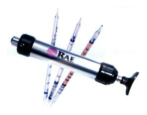
**RAE Systems hand pump** is easy to use with a rugged metal construction.
