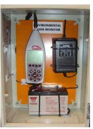
The kit contains all necessary masts, windscreens, cables, battery packs and adapters required for use with the SoundPro Real-Time Analyzer.
