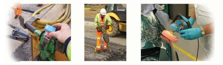
THE HAVMETER GIVES POWER TOOL USERS A RUNNING TOTAL OF THEIR VIBRATION POINTS EXPOSURE THROUGHOUT THE DAY AND WARNS BEFORE HIGH EXPOSURE LEVELS ARE REACHED.
