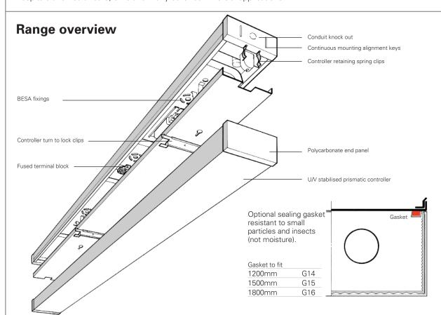
The FT400 single and twin lamp batten-type luminaires are strongly constructed from from zinc coated steel sheet. Finished in durable gloss white epoxy polyester as standard, other colours may be supplied to special order.
