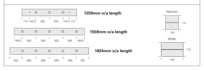
This robust and versatile surface luminaire range is ideal for education, health care, civic and commercial applications. Two body widths, firmly fixed diffusers or reflectors and the ability to mount continuously offer many lighting options. Available for T5 or T8 lamps with dimmable and integral emergency conversions if required.
